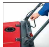
Lever for raising / lowering side brush
