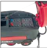
Machine open showing the batteries
