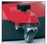
Guide wheel with brush pressure adjusting screw
