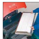
The filters can be changed without tools.
